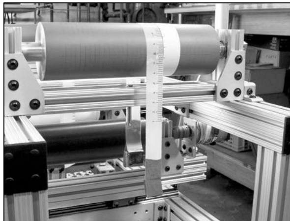
Figure 2 – Microslip experiment on a static roller
