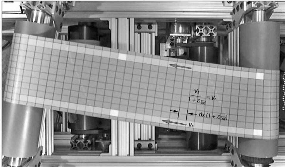
Figure 3 Qualitative Demonstration of the Velocity-Strain equation.
