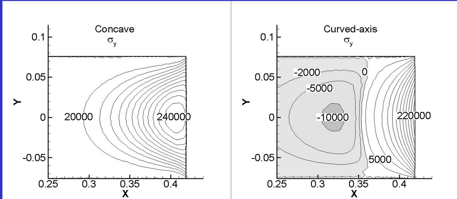
The rollers show similar patterns of cross web stress at the downstream roller. The curved-axis spreader shows a region of compressive stress (shaded). But, levels are low. There is a similar pattern for the concave roller that is just beyond the area shown in the graph. It has a peak value of  $-825$  Pa.
