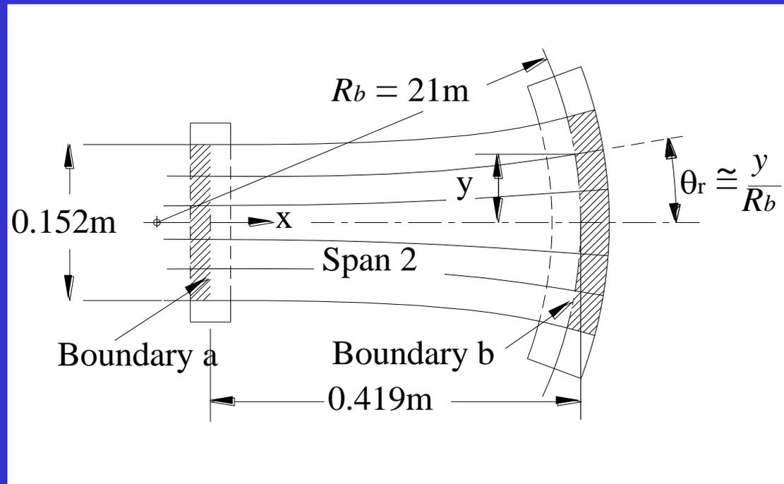
Curved-axis roller using same span parameters as Markum and Good experiment.
