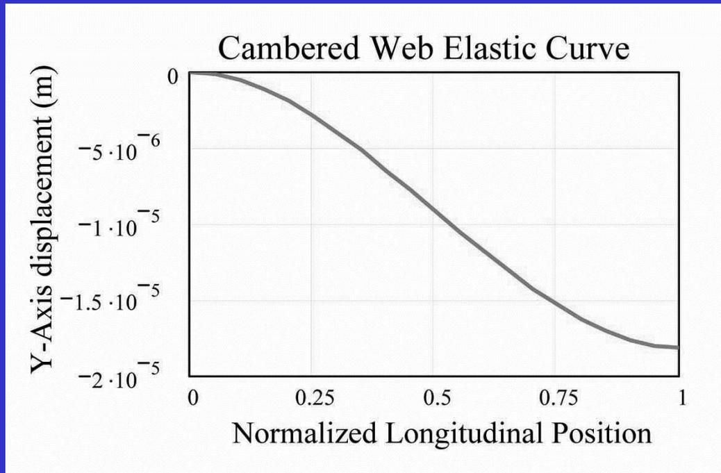
Plotted relative to a horizontal line through the center of the web at the upstream roller.
