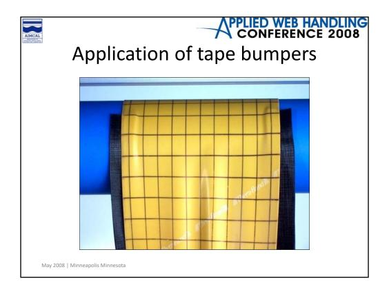
After twisting the web 45 degrees, tape bumpers were introduced in a way that didn't alter the initial conditions. The bumpers had to be 1/16 inch thick to prevent wrinkles.
