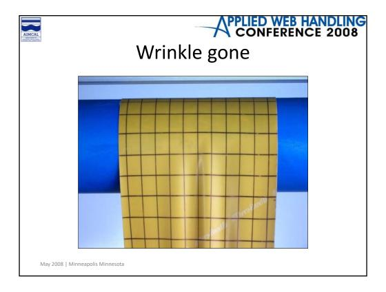
Notice that the horizontal black lines are frowning. Without traction, the normal entry rule can't operate.
