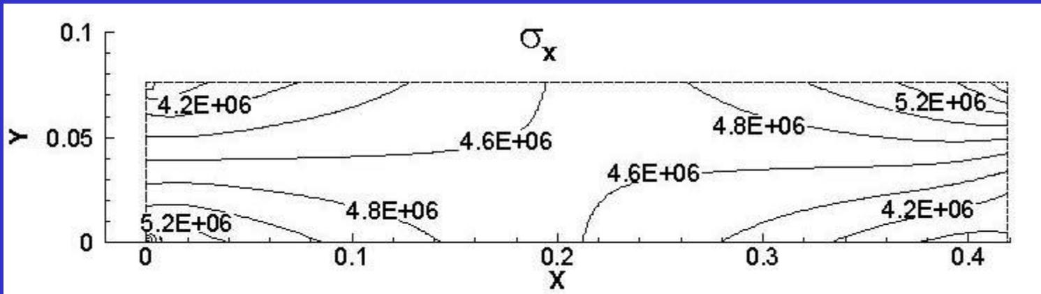
There is a nice symmetry in the  $\sigma_x$  field. A plot of the displacement would show that this is because the deformed web has a symmetrical “s” shape. Stresses are in Pascals.
