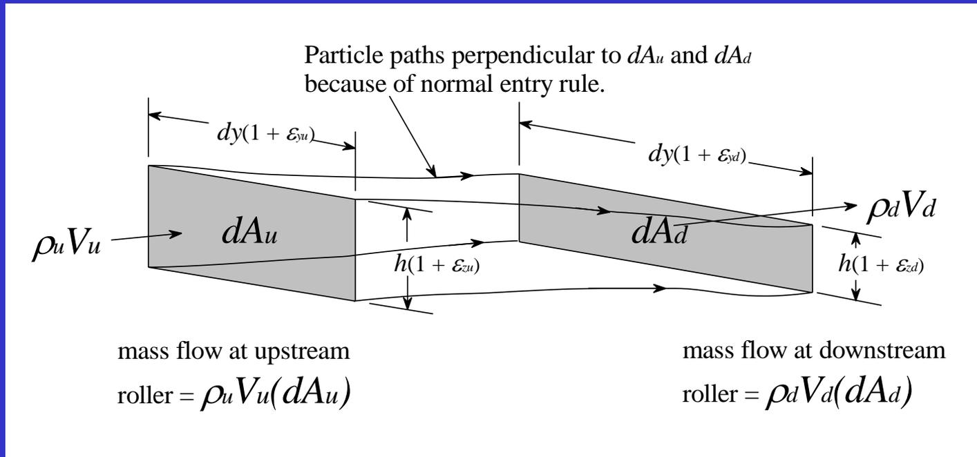
Start by considering the mass flow at upstream and downstream rollers through increments of width that were equal to  $dy$  in the relaxed web. The mass flows must be equal. However,
